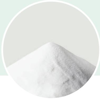
MECELLOSE®, environmentally friendly, uses cellulose as a primary source, which can be obtained from wood or cotton. Cellulose is a water-insoluble natural polymer that has 30~65% crystallinity formed by hydrogen bonds between molecules. Through a chemical process called 'Etherification', this water-insoluble cellulose is turned into water-soluble nonionic cellulose ether, MECELLOSE®.
