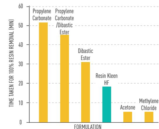
For a procedure in which polyester resin was coated onto aluminium strips, partially cured for (12 hrs) and submerged in a beaker containing the respective formulations, at ambient temperature in the absence of agitation (experiment covered under patent U.S. P. 6,187,108).
