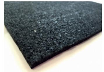
Protection Mat is made up of natural and synthetic elastomeric compounds and has a density of 950 kg/m<sup>3</sup>. It is manufactured from recycled materials with one of the main components being recovered PFU (from used car tyres), bound by polyurethane resin.
