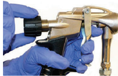
Image 4: Black valve to adjust spray pattern.
