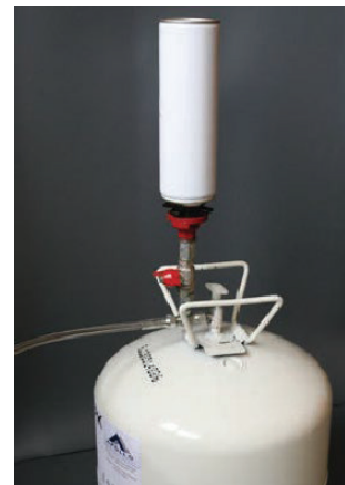
Image 10: Screw Cleaning Aerosol into the adaptor
