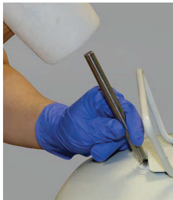
Image 17: Pierce disk at perimeter
