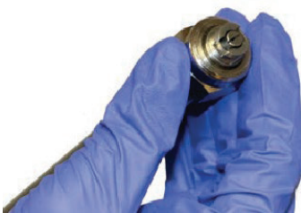
Image 3: Attach the spray-tip
