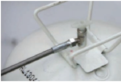
Image 1: Canister with the braided-hose attached properly.
