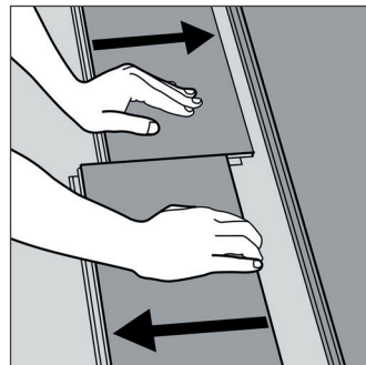
Fig 12. Disassemble the panels by sliding horizontally.
