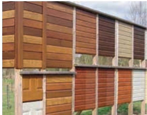
Testing Teknos on Accoya® cladding compared with other timber species.
