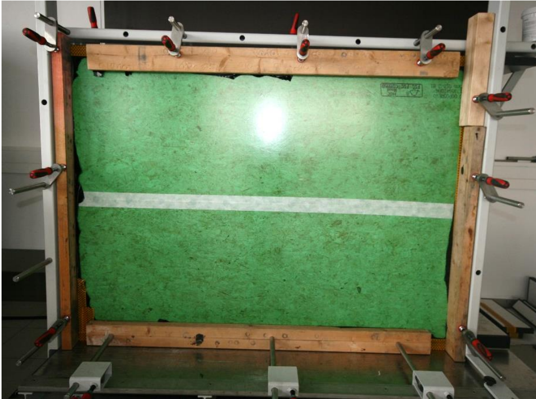
Image 3: Two adjacent OSB panels, joined with tape in the test facility
