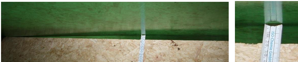
Picture 4: Deformation of the panel @ 2000 Pa, deflection of about 2 cm at a span of 1600 mm. The second panel in the front is used as a reference to measure the deflection.
