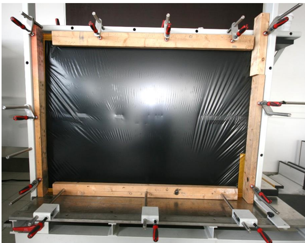
Image 2: Two adjacent OSB panels, joined with tape in the test facility and covered with the membrane to enable measurement of the air tightness of the test facility
