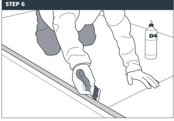
All exposed edges should be sealed by applying a continuous layer of D4 rated (EN 204) adhesive by using a brush or by wrapping a specialist waterproof high-performance polyethylene-coated cloth tape around the edges.
