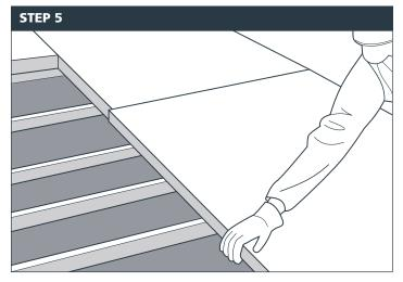
Continue installing the panels as required in a staggered pattern by repeating the fixing, gluing and taping steps for each panel.
