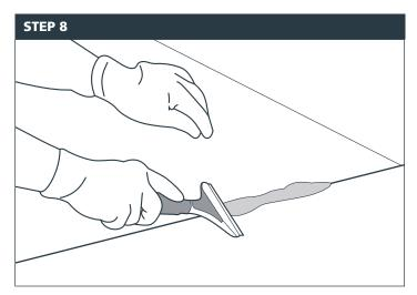
After any construction work has been completed the floor should be cleaned. The expanded foam should only be removed with a scraper when the building is weathertight to prevent water ingress and edge swell.
