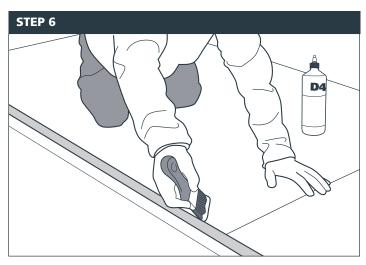
All exposed edges should be sealed by applying a continuous layer of D4 rated (EN 204) foaming adhesive by using a brush.
