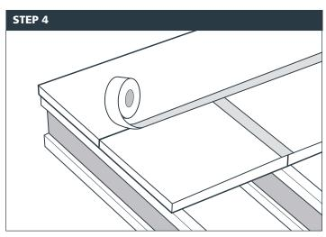
All floor joints should be sealed and protected with a specialist waterproof high-performance polyethylene-coated cloth tape. This will prevent moisture ingress in the panel edge and edge swelling.
