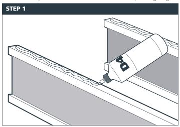
Apply one continuous bead of D4 rated (EN 204) foaming adhesive to the top of the joists and noggins corresponding to the area of the 1st panel to be installed.
