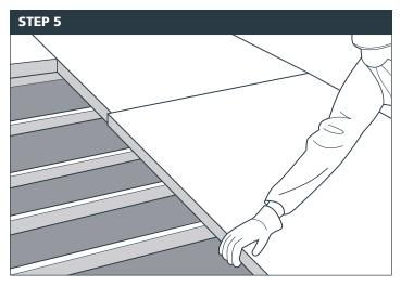
Continue installing the panels as required in a staggered pattern by repeating the gluing and fixing steps for each panel.
