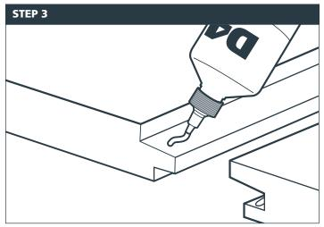
Apply one bead of D4 rated (EN 204) foaming adhesive on both the tongue and groove of the joints about to be installed making sure that the entire joint is bonded. The adhesive should foam out of the joints on the panel surface once installed to help seal the joint and prevent water ingress and edge swelling.
