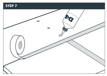
Fixing heads should be sealed by applying a bead/drop of D4 rated (EN 204) adhesive or by tape.
