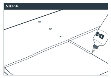
Apply one bead of D4 rated (EN 204) foaming adhesive on the cut edges on top of the joists allowing the adhesive to foam out on the panel surface to help seal the joint and prevent water ingress and edge swelling.
