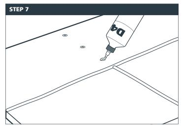
Fixing heads should be sealed by applying a bead/drop of D4 rated (EN 204) foaming adhesive.
