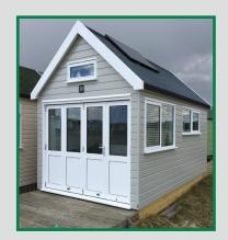
MEDITE TRICOYA EXTREME provided the high performance, water-resistant cladding to ensure a stunning and exclusive set of beach huts retained an attractive exterior despite the climactic rigours of a seaside location.
